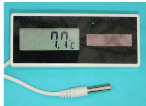
The module has an external probe fitted, which is 50mm long and 8mm diameter (6mm at the tip). The probe is supplied connected to 3m of cable. The external probe should be fixed in the same pocket as the NTC sensor. If it is necessary to extend the cable this should be done using the minimum possible length of cable as long runs causes a decrease in accuracy.
