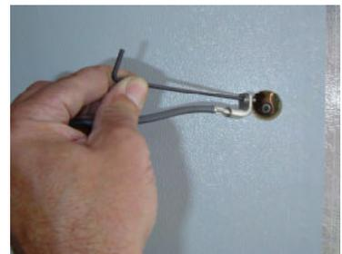
It is recommended that sensor cable connections are made using insulated crimps, rather than junction boxes as these provide long term low resistance joints.
