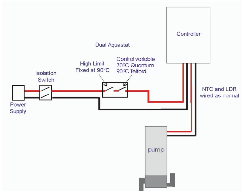
**B3 Figure 9:** Schematic electrical diagram of dual aquastat.
