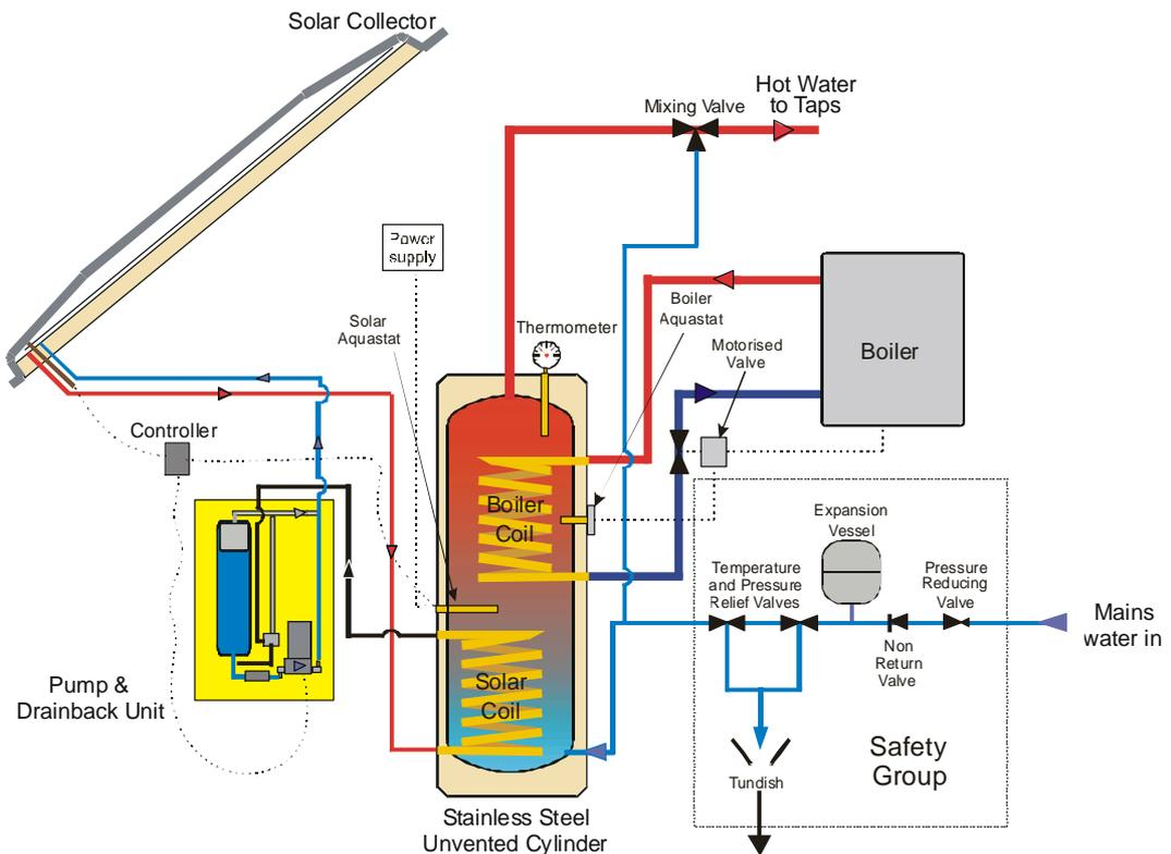
**B3 Figure 8:** A mains pressure (unvented) system. The system must be fitted with the safety devices. Note that the return from the panel is connected to bottom of solar coil so the direction of flow is upwards through a 22mm coil (see section B3.2 on connecting to a large diameter coil).
