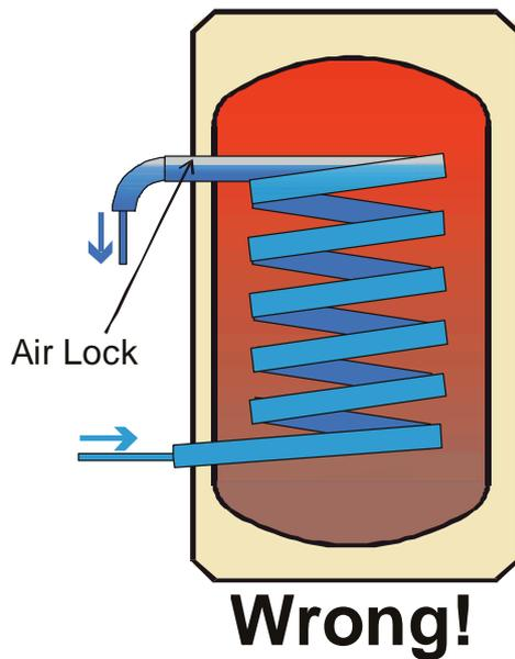
3. The top connection to the solar coil (flow out of coil) should have a 22mm elbow fitted facing upward, before being reduced to 8mm or 10mm microbore. This prevents small air pockets being formed in the top of the coil which will cause an airlock and prevent drainback.
