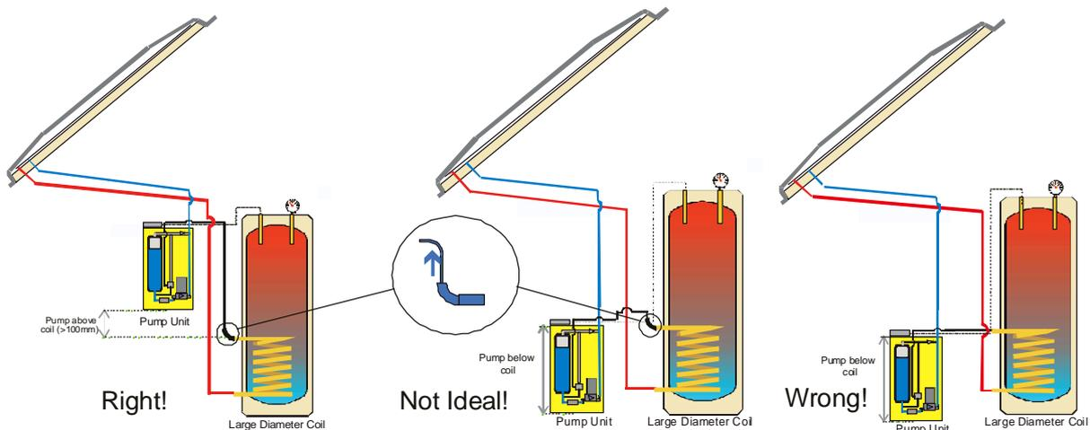
**B3 Figure 2:** Drainback unit positioning with a large diameter solar coil: DBU should be higher than solar coil.
