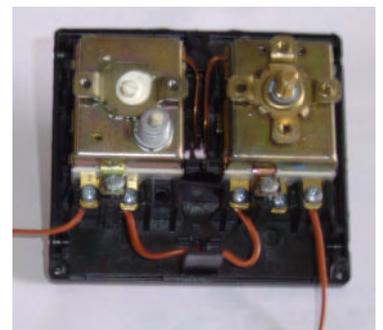
**B3 Figure 10:** Practical wiring diagram of dual aquastat.
